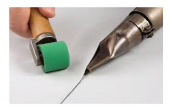
Another common mistake is applying heat, removing the heat, then getting the roller and applying pressure without the Leister still being directed at where your roller is working.
