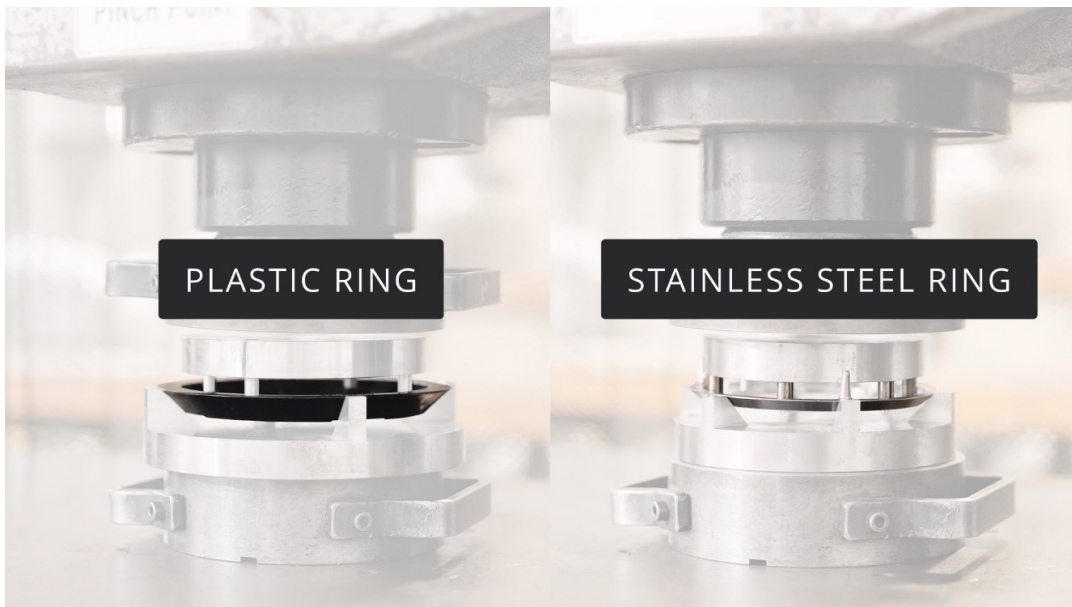
Clamping Rings mounted into the test machine
